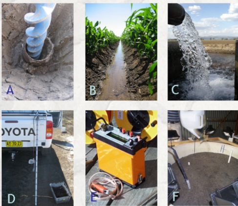
Fig.1a: hand augering holes for resistivity probes Fig.1b: flood irrigation of cracked soil Fig.1c: irrigation water at pump outlet Fig.1d: Resistivity probe before installation in the field Fig.1e: ABEM resistivity meter for electrical resistivity tomography Fig.1f: Tracer application on soil column during resistivity tomography measurements
